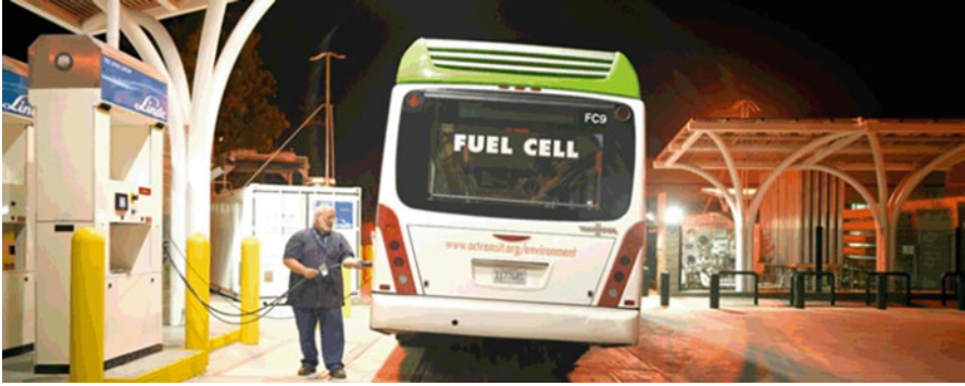
Fig. 5.15 Bus with fuel cell drive functionality at a hydrogen fuel station. (Courtesy of Linde Group)
