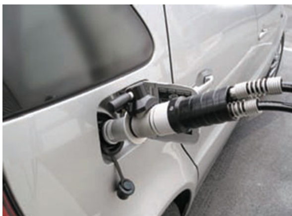
Fig. 1.22 Hydrogen fueling nozzle. (Courtesy of the US Office of Energy and Renewable Energy)
