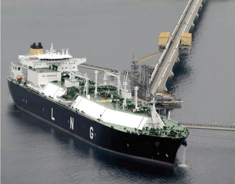
Fig. 4.3 130,000 m 3 liquid natural gas (LNG) carrier with integrated Invar tank
