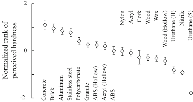
Fig. 4. Subjective hardness scores of the specimens, including the means and standard errors of the scores among the participants (modified from [8])
