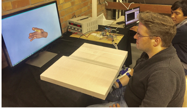
Fig. 5. The experimental setup. In this experiment participants were asked to wear the ExoTen-Glove and squeeze a set of virtual springs with different stiffness by their thumb and index finger while the ExoTen-Glove were covered.
