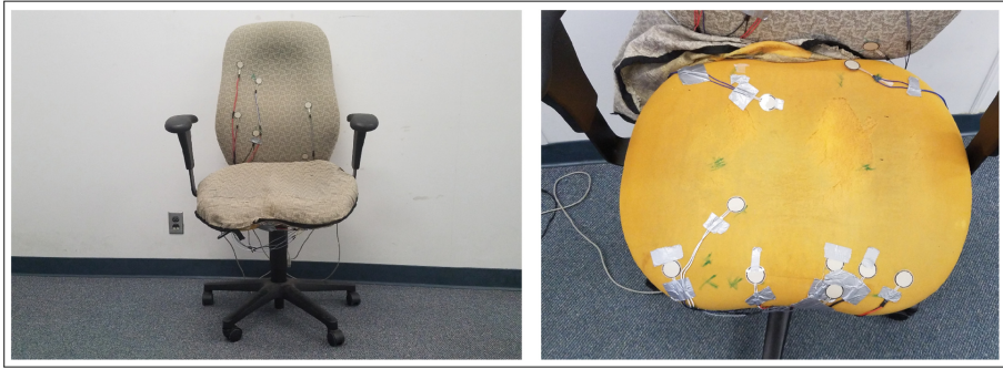
Fig. 1. Assentiation prototype chair: (a) as seen by the user, and (b) uncovered seat-bottom sensor placements.
