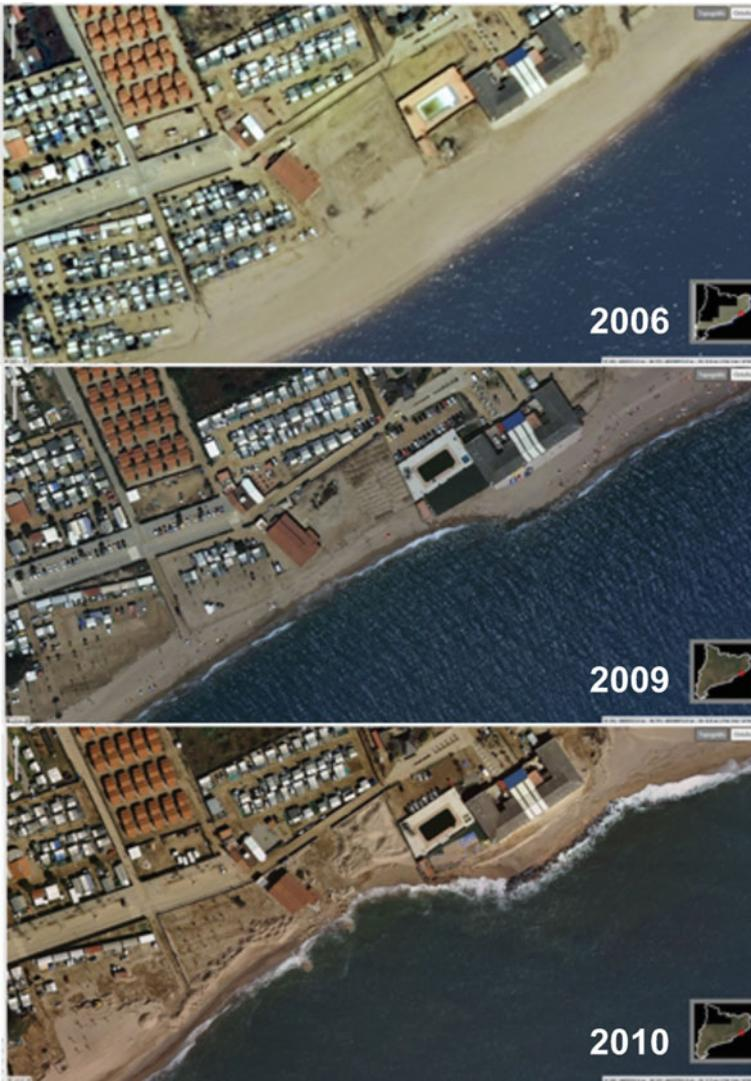
**Fig. 32.8** Downdrift induced erosion due to a revetment built in front of a campsite in the northernmost part of the Maresme coast
