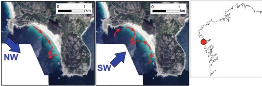
**Fig. 9.5** Variations in the exposed beach of Louro at the west coast. The most common longshore transport is southward, but with SW storms the beach develop two cells forcing a northward transport in the south end of the beach (after Almécija et al. 2008)
