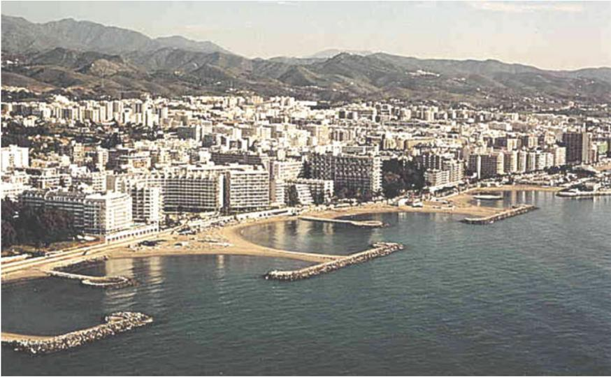
**Fig. 13.15** Frequent layout of hammerhead groyne fields in Malaga's beaches in 1970s. Photo of Marbella in 1974. *Source* Ayuntamiento de Marbella Archivo
