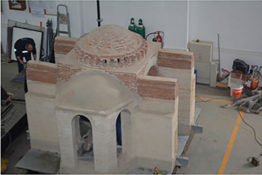
Fig. 7.6 Scaled model of Hagia Sophia on the shake table
