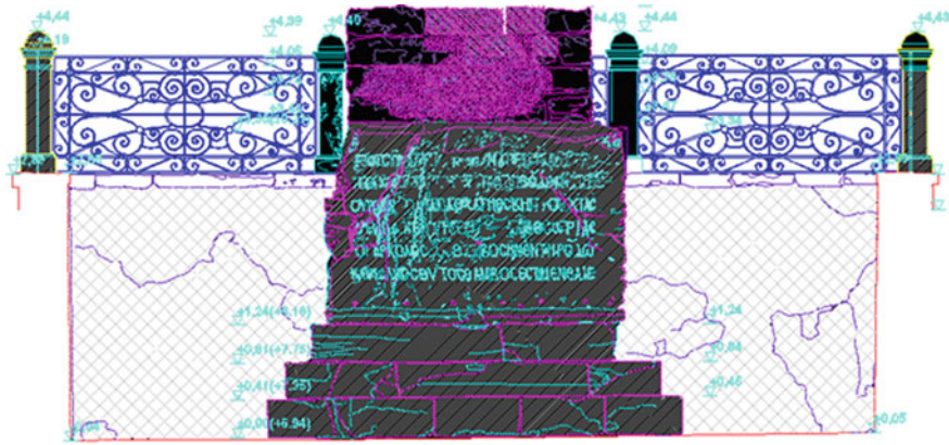
Fig. 3.4 Illustration of the residual displacement at the bottom of the “Walled Obelisk” monument in Istanbul in December 2008. The massive stone surface was shifted above the level of 1.24 m, which is not entirely the original position (Kasimzade et al. 2011)
