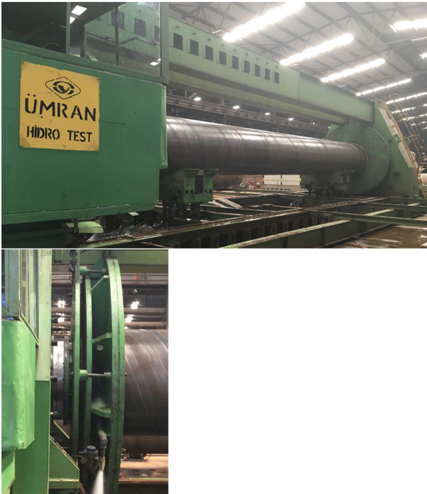
Fig. 12.4 Hydrostatic test setup
