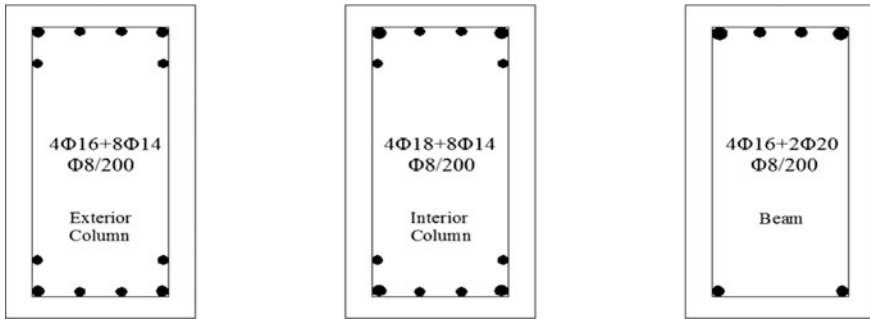
Fig. 17.4 Section details of columns and beams
