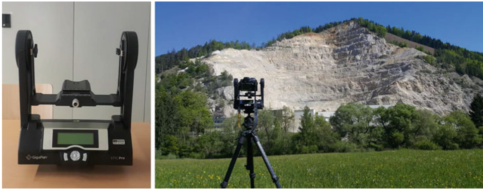
Fig. 2 GigaPan epic pro robotic mount (left) and instrument set-up at the dolomite quarry (right)
