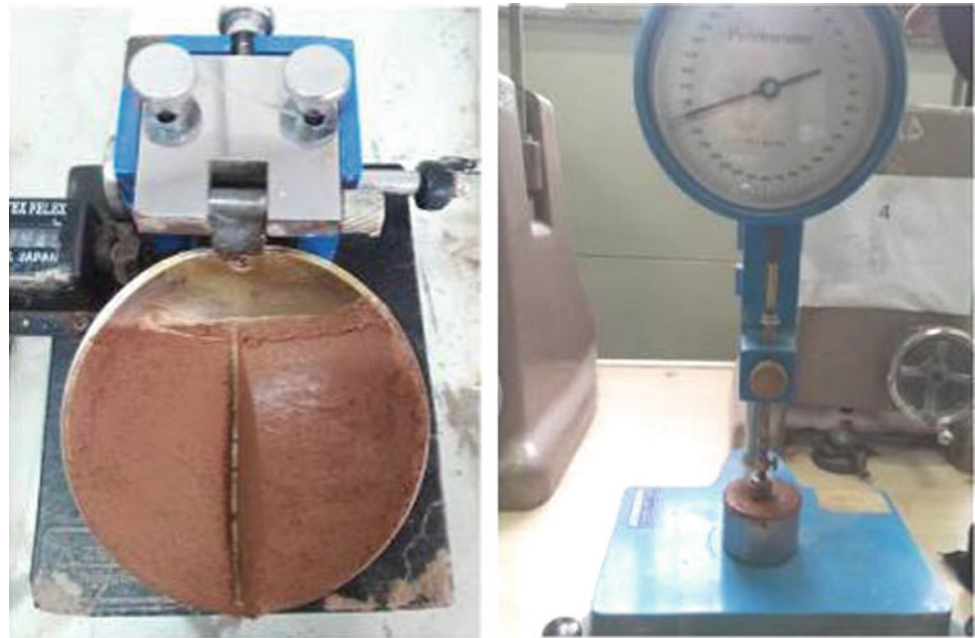
Fig. 3 The Casagrande apparatus (left) and the fall cone apparatus (right)
