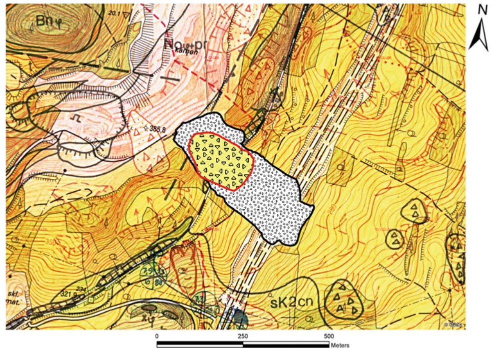
Fig. 3 Cut-out of the engineering geological map manuscript (Pašek and Janek 1972) with the already known partial landslide (red) approximately in the area of the future slide of Dobkovičky (black) geo-referenced over the map of 1:10 000 scale with the apparent course of the motorway
