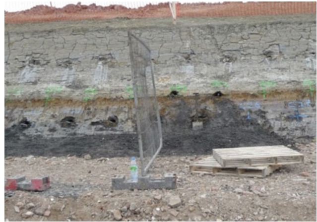
Fig. 5 Jurassic Oxford Clay strata comprising weaker soil like mudrocks with discontinuous nodular limestone beds
