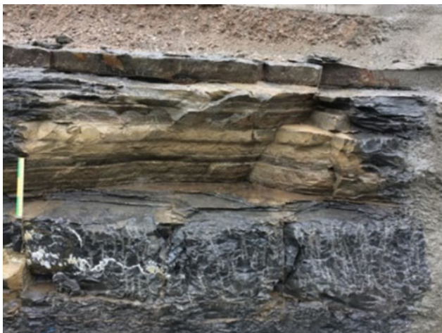
Fig. 11 Water flow from limestone horizon interbedded with mudstone
