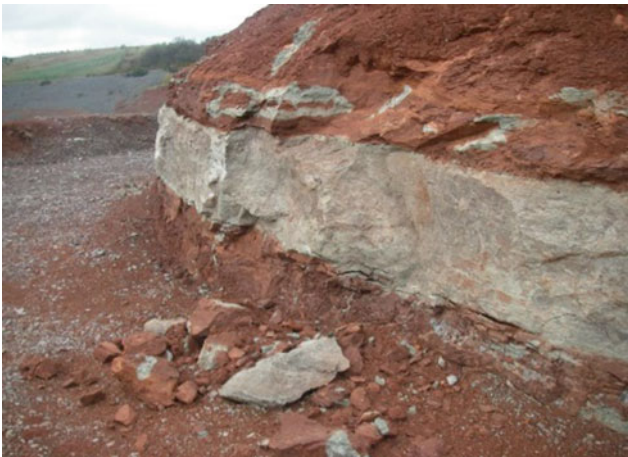
Fig. 3 Mercia Mudstone strata comprising argillaceous red-beds and light grey fine sandstone skerrie bed showing instability
