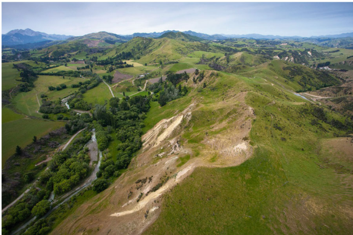
Fig. 4 Landslides and surface rupturing faults at Glenbourne Farm, Hurunui District. Top: Orthophoto showing the fault rupture (red). Areas of major slope movement are numbered. 1: incipient failure, open fissuring and dilated rock mass. Fissures subparallel to the fault traces.
