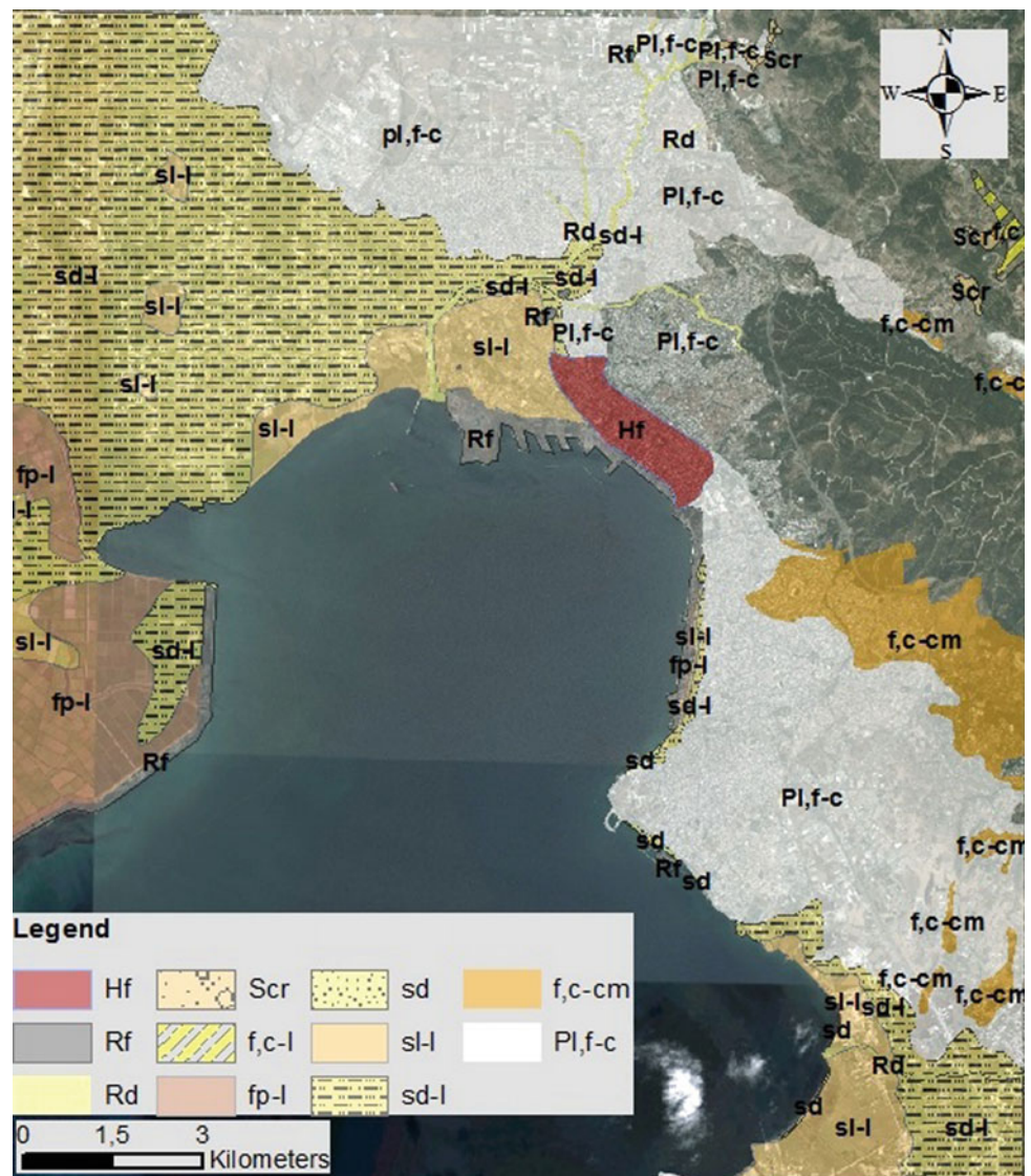
Fig. 1 Engineering geological map of Thessaloniki (modified by Rozos et al. (2004)). Coastal sands (sd), torrential deposits (Rd), inland basins deposits (f,c-l), Quaternary loose sandy deposits (sd-l), Quaternary loose silty deposits (sl-l), Quaternary loose fine deposits with organics (fp-l) Quaternary scree material (Scr) and the Pleistocene cohesive sediments of mixed phases coded as f,c-cm
