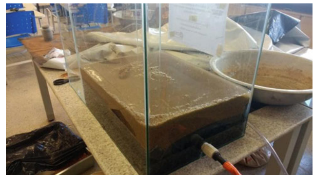
Fig. 4 Apparatus for carrying out the quicksand phenomenon
