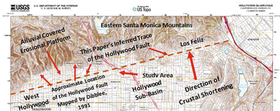
Fig. 4 Suggested trend of the Hollywood Fault following regional geomorphic features and perpendicular to the direction of crustal shortening
