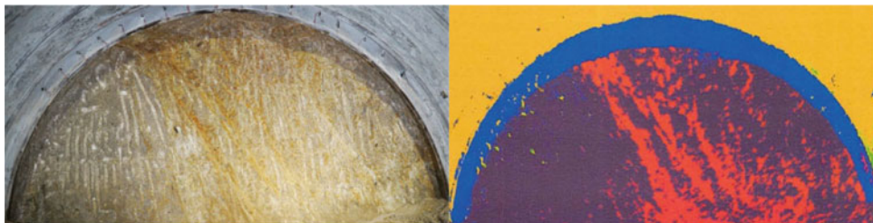
Fig. 6 Tunnel face image by RGB color model (left) and its weathering evaluation by hyper-spectral camera (right)
