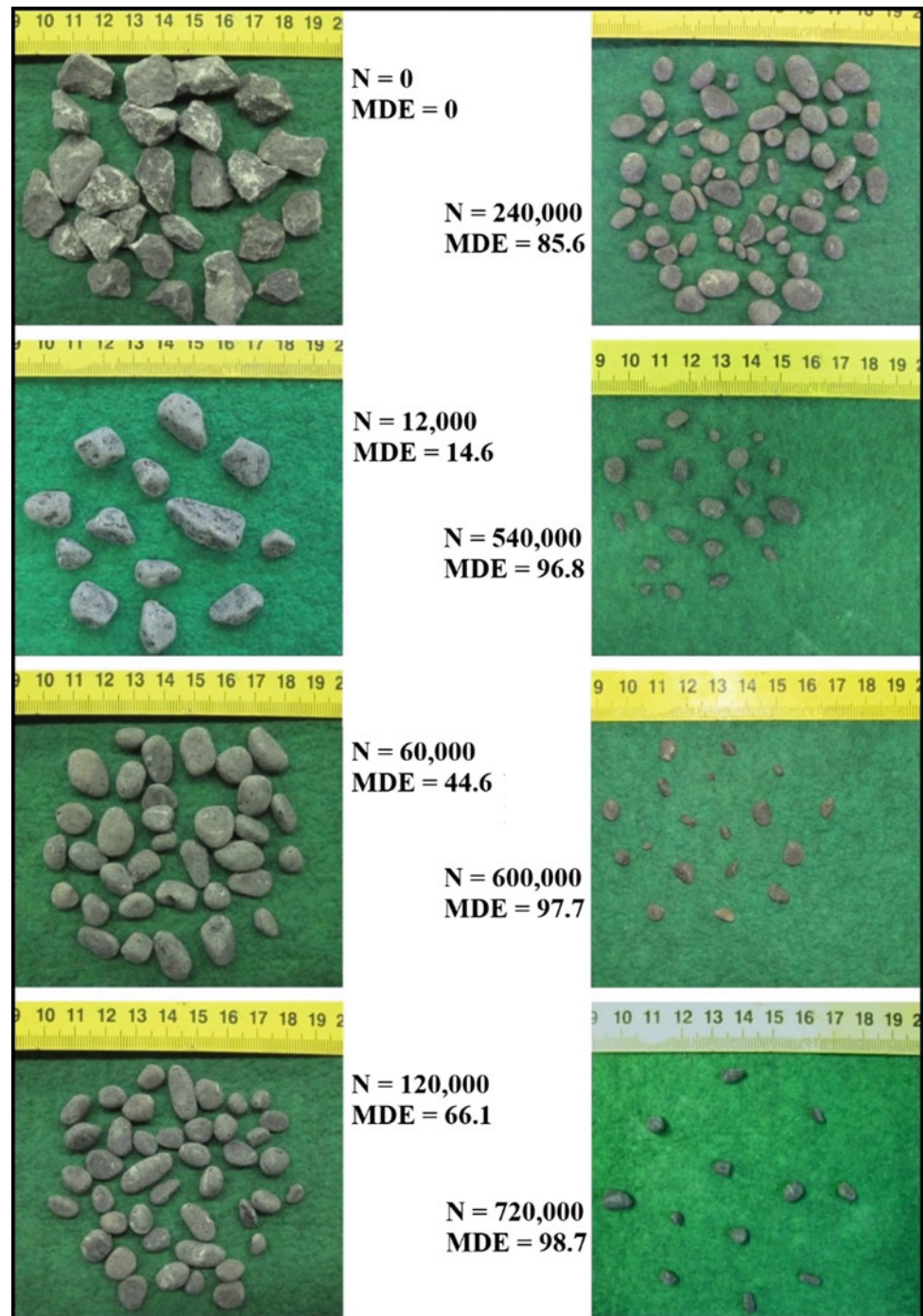
Fig. 2 The grains of the aggregate samples during the long-term Micro-Deval tests (N: number of rotations, MDE: Micro-Deval value)
