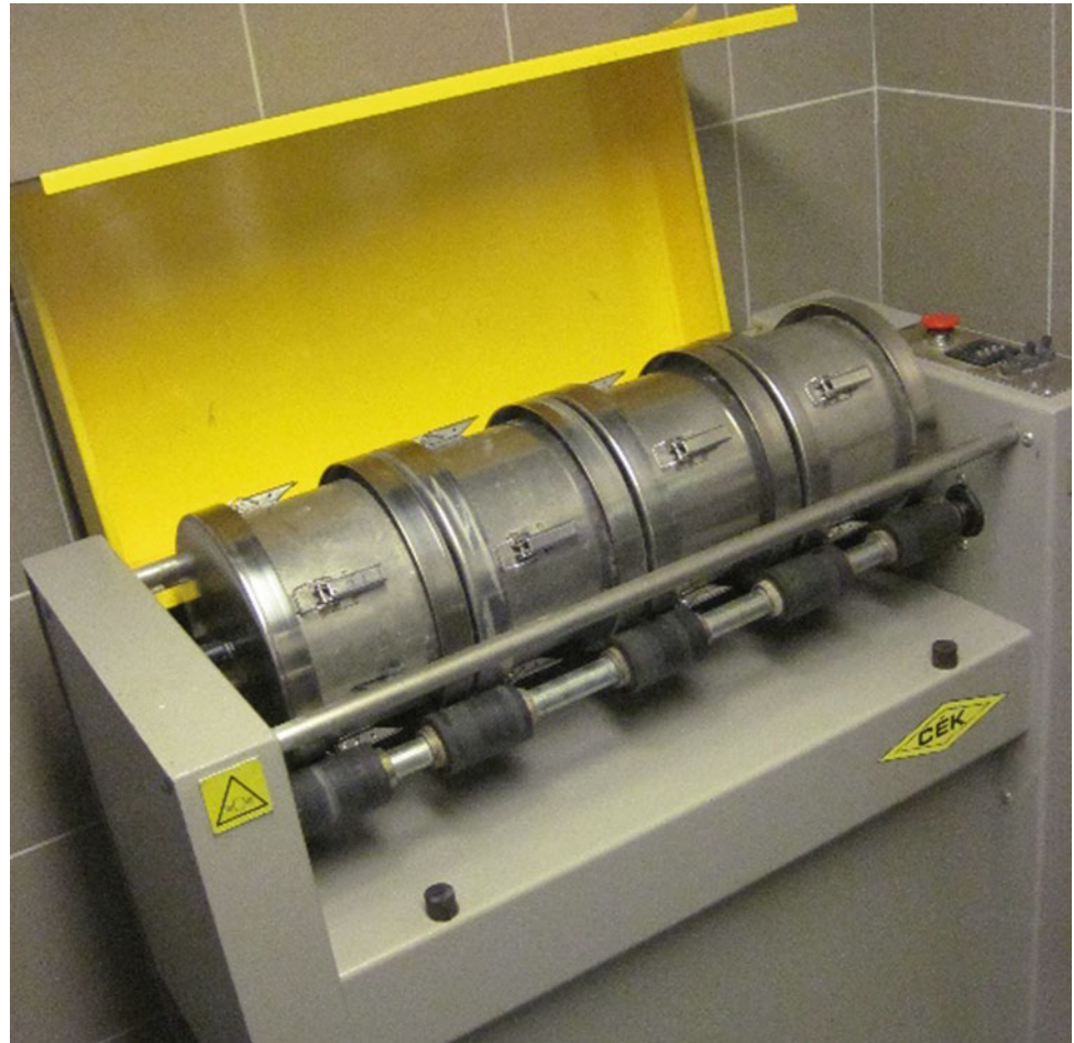
Fig. 1 The Micro-Deval test machine with four steel drums
