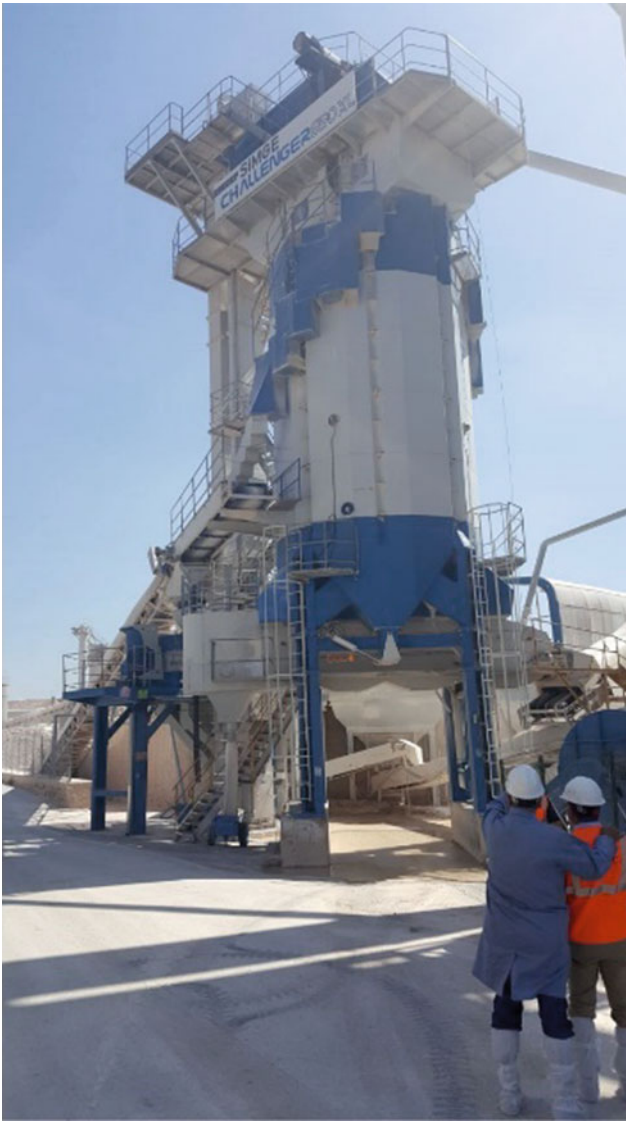
Fig. 8 A closed aggregate preparation system
