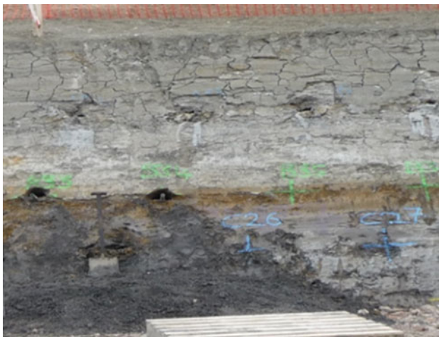
Fig. 11 Colour changes clearly evident in a weathering profile affected by pyrite oxidation seen in Oxford Clay
