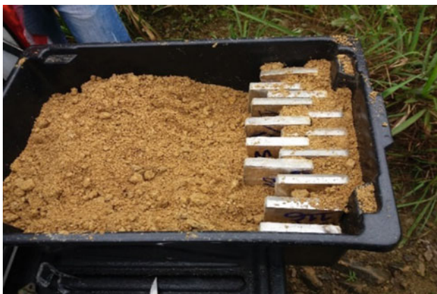
Fig. 2 Metal molds to the drained shear test
