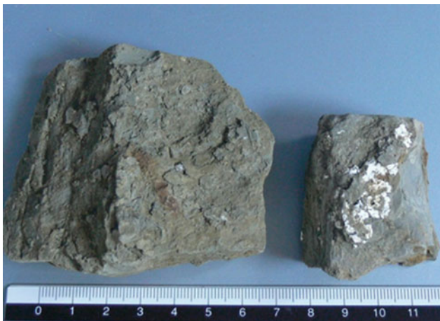
Fig. 9 Oxidation of pyrite forming selenite observed in sample on right during stages of Slake Durability Testing
