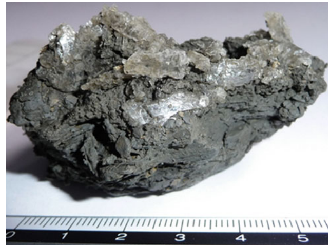
Fig. 7 Development of randomly orientated selenite crystals within a weak soil-like mass of Lower Lias Clay
