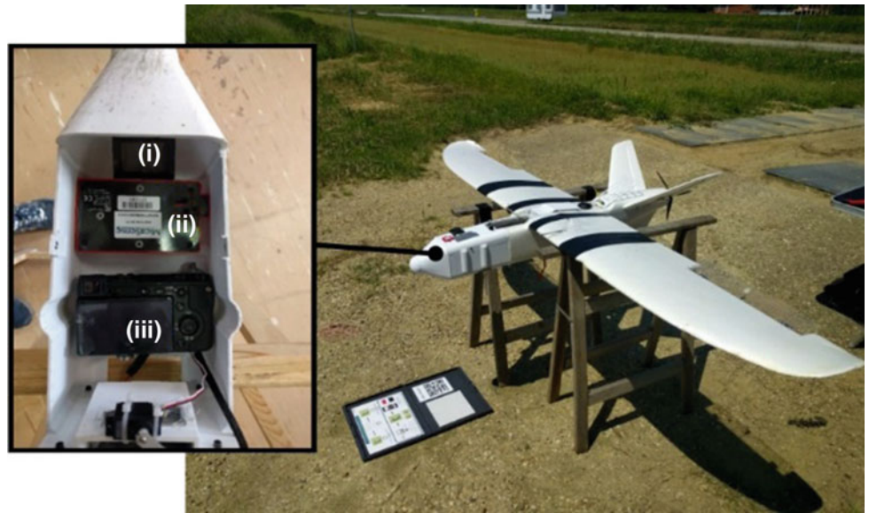
Fig. 3 CNR IRPI fixed wing drone with onboard mounted sensors: (i) action camera, (ii) multispectral camera, (iii) RGB mirrorless camera
