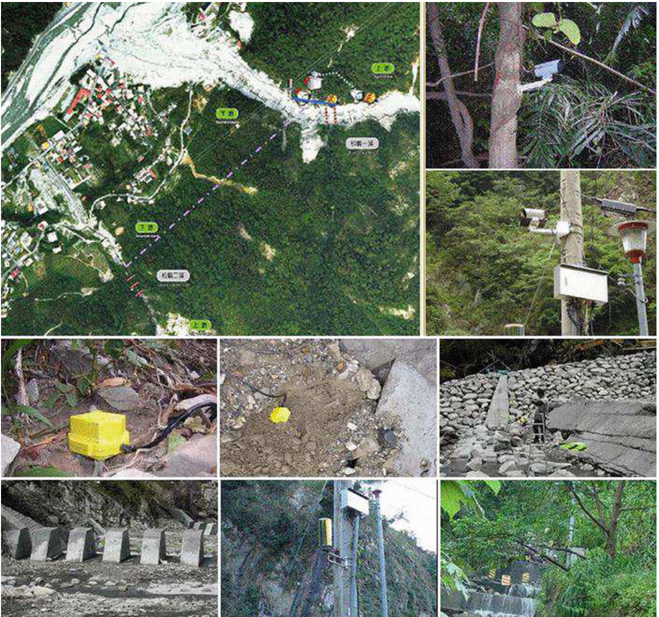
Fig. 6 The equipment at the Songhe Debris flow monitoring station includes 1 rain gauge, 2 CCD cameras, 2 geophones and 8 wire sensors
