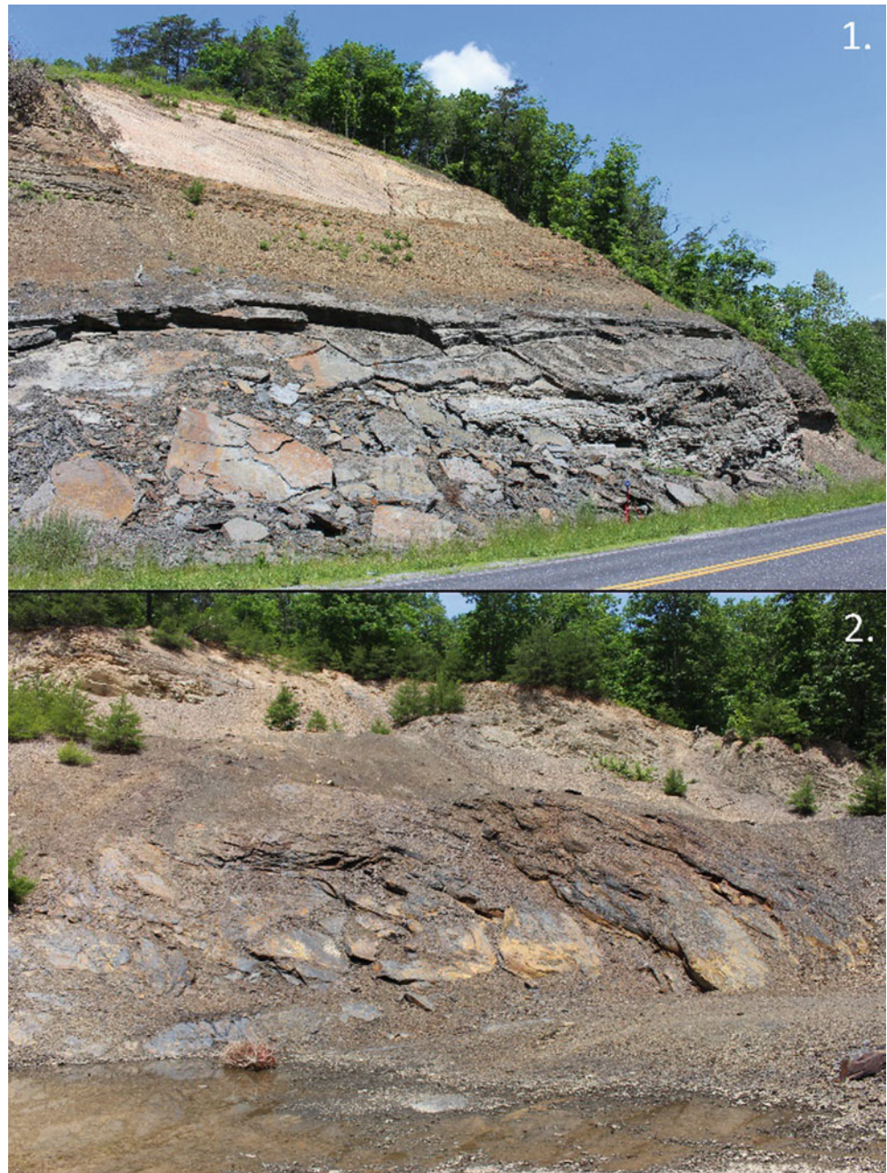
Fig. 2 Top image: Deerfield site, facing the cut slope from the left portion; general bedding orientation dips 20^\circ towards 280^\circ , view bearing is roughly 350^\circ . Bottom image: Cove Mountain site facing the pit slope; general bedding dips 10^\circ towards 300^\circ , view bearing is roughly 30^\circ . Photos taken by author, 2016
