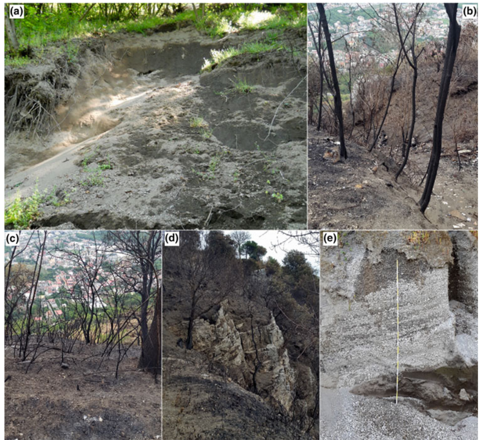
Fig. 2 Field surveys photos: a Landslide main scarp and deposit; b burnt trees and stream; c burnt trees and Palma Campania inhabited area in the background; d burnt vegetation and limestone outcrop in the background; e pyroclastic deposit
