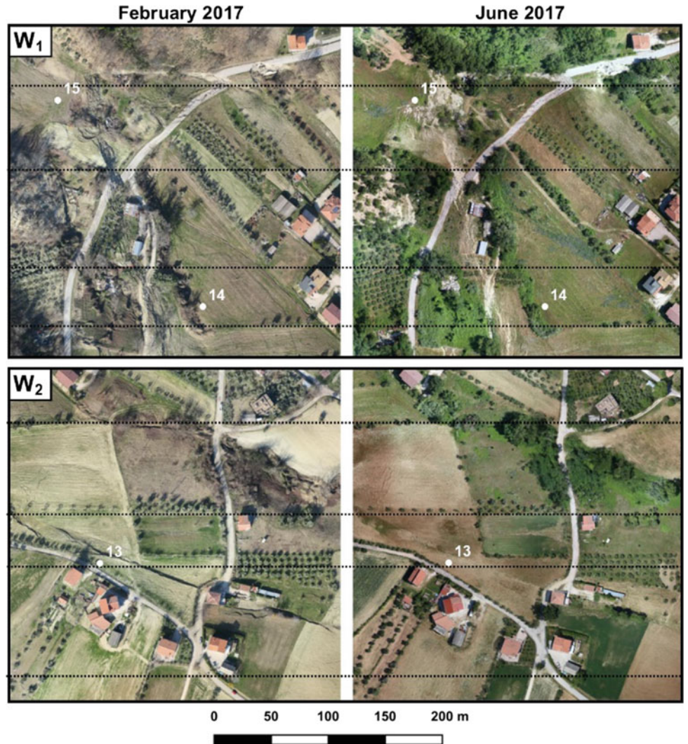
Fig. 4 Comparison of a small part of UAVs aerial surveys performed in February and June. The geographic location is shown in Fig. 2. The horizontal lines are reference lines to aid a multitemporal comparison
