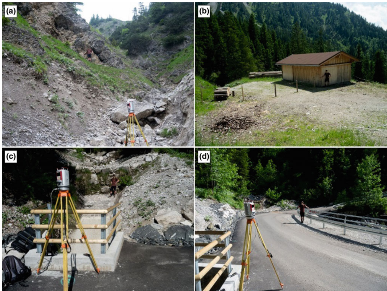
Fig. 3 Areas without geomorphic change in the study area used for registration of the point clouds. a Rock face in the topmost part of the channel; b shed and its near range in the middle part of the channel; c, d drainage and street in the lowermost part of the channel
