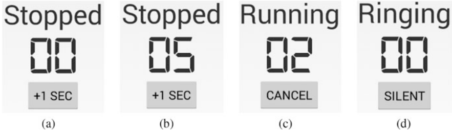
Fig. 6 View states for the countdown timer. (a) Initial stopped state with zero time. (b) Initial stopped state after adding some time. (c) Running (counting down) state. (d) Alarm ringing state
