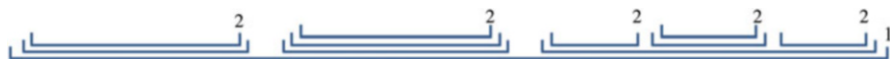
Fig. 10 Resource of parallelism of a program: parallel loops are marked by ‘1’ or ‘2’ in the loop profile of the program
