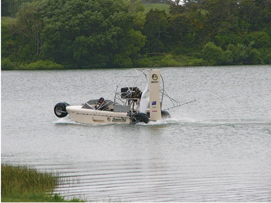
Fig. 7.13 Spraying alum onto the surface of Lake Okaro. The airboat was fitted with GPS navigation to control where the spray was applied [photo by M. Gibbs, NIWA]
