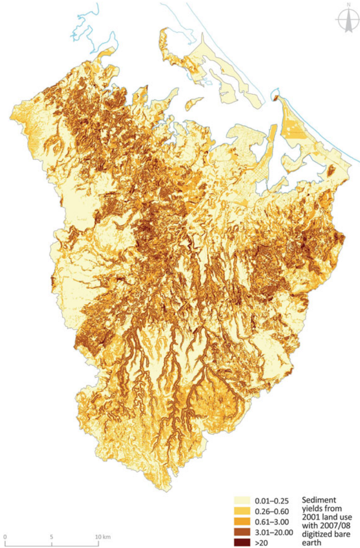
Fig. 2.4 Sediment yields (tonnes/ha/y) for the current land use, mapped for every 30 m × 30 m model cell (over 1.1 million cells in total), estimated using GLEAMS
