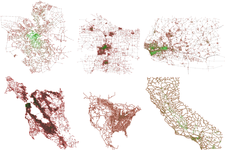
Fig. 5. Visualizations of real-world road networks of Oldenburg (top-left), San Joaquin (top-mid), Le Havre (top-right), San Francisco (bottom-left), USA (bottom-mid), California (bottom-right). Green color indicates nodes of high reliability score. (Color figure online)
