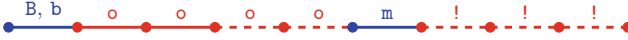
Fig. 1. Representation of X = \{\mathbf{B}, \mathbf{b}\}^{1,1} \{\mathbf{o}\}^{2,4} \{\mathbf{m}\}^{1,1} \{\mathbf{!}\}^{0,3} . Each string of \gamma(X) starts with \mathbf{B} or \mathbf{b} , followed by 2 to 4 \mathbf{o} s, one \mathbf{m} , then 0 to 3 \mathbf{!} s.
