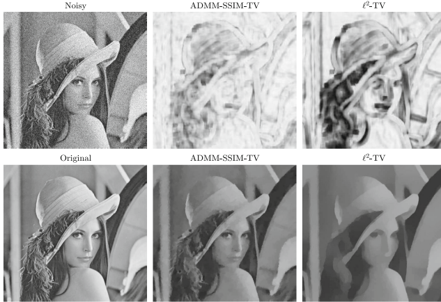
Fig. 1. Some visual results for the denoising of the test image Lena . The TV seminorm of both reconstructed images is 2500. Top row: Noisy image along with SSIM maps between each reconstructed image and the original. Bottom row: Original and ADMM-SSIM- and \ell^2 -based denoised images, with MSSIM values 0.6468 and 0.4386, respectively.
