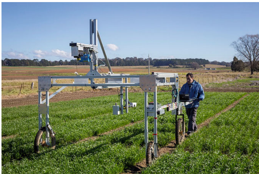
Fig. 7.3 A ‘Phenomobile Lite’ carrying sensors above a wheat trial, a noninvasive method to phenotype cereals in situ. HRPPC CSIRO Canberra, Australian Capital Territory
