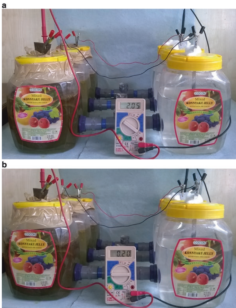
Fig. 10.1 (a) Voltage production of MFC connected in series. (b) Current production of MFC connected in series
