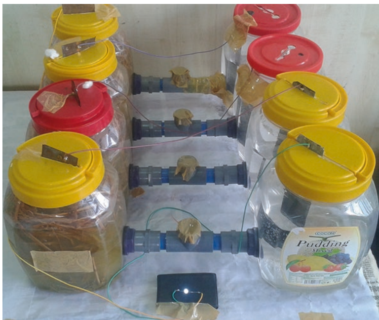
Fig. 10.10 Rumen fluid MFC glows a 1.5 \text{ V} white LED
