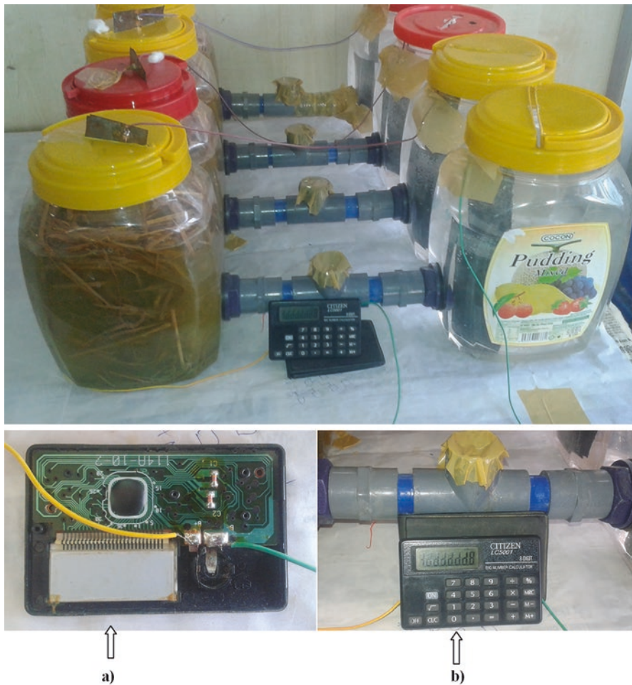
Fig. 10.11 MFC powering a pocket calculator. (a) Calculator soldered with the positive and negative ends of MFC. (b) Calculator getting powered by MFC
