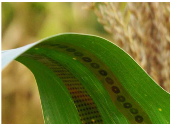
Fig. 3 Plant sensors for direct measurements of water use in crops [7]
