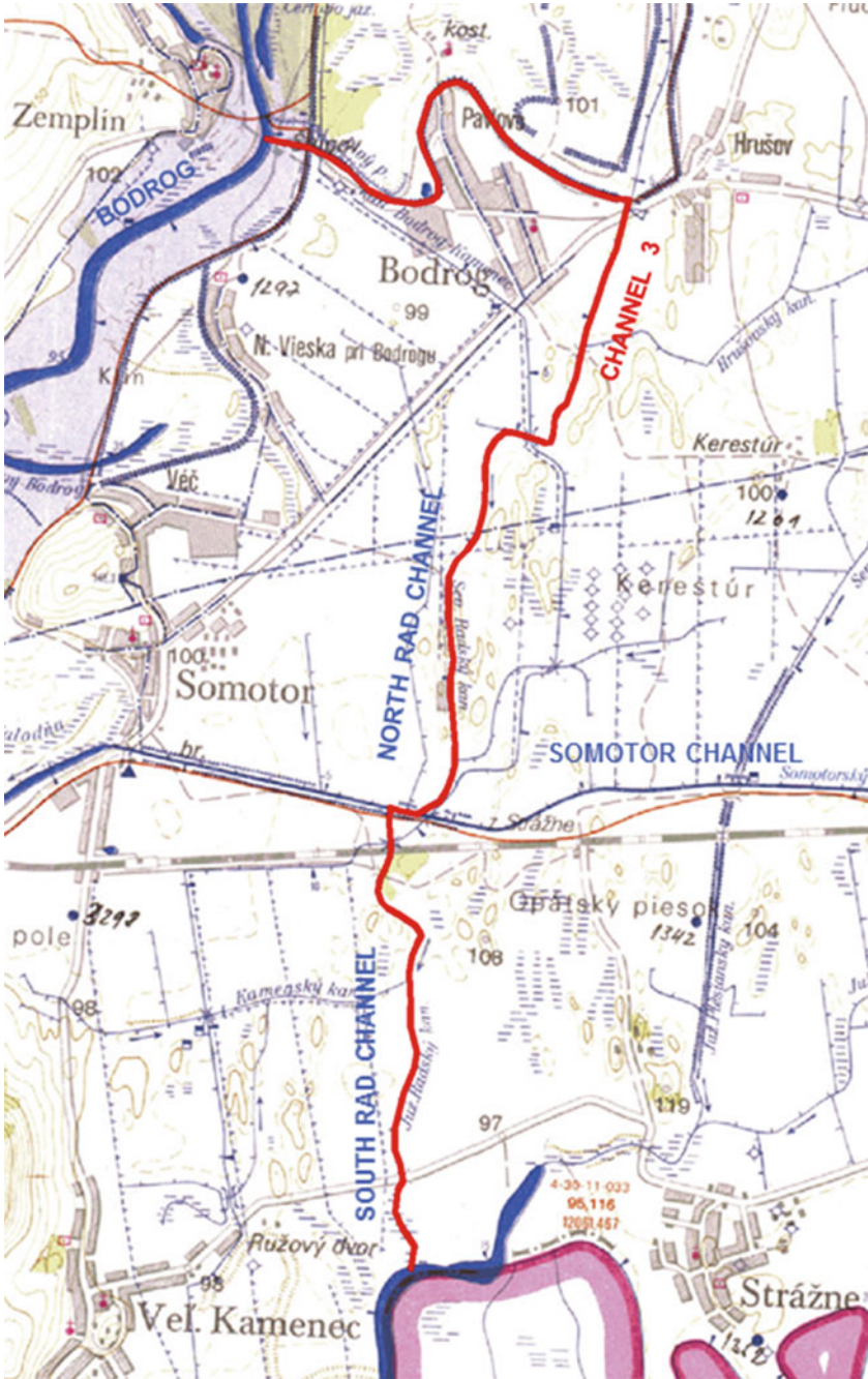
Fig. 8 Southern branch of the water connection from the Tice River through the Radský channel into the Krčava River
