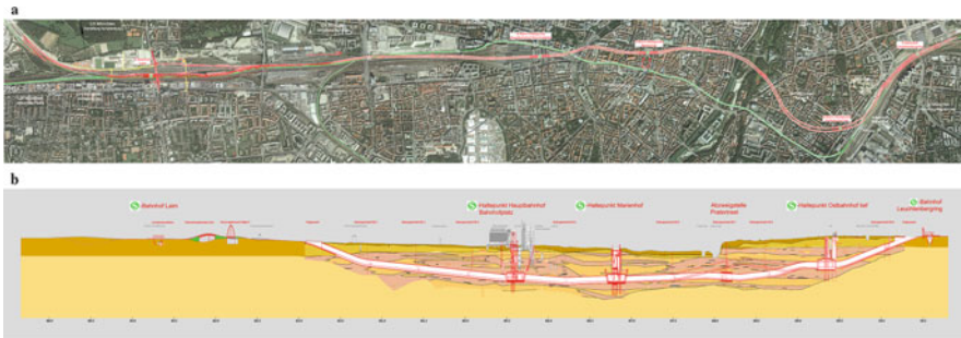
Fig. 32.2 (a, b) Location and elevation plan for the second principal rapid transit line (red) in Munich with the planned stations Hauptbahnhof, Marienhof and Ostbahnhof. (© OBERMEYER Planen + Beraten, reprinted with permission)
