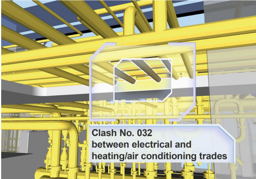
Fig. 30.6 Clashes between technical building services. (© HOCHTIEF ViCon, reprinted with permission)
