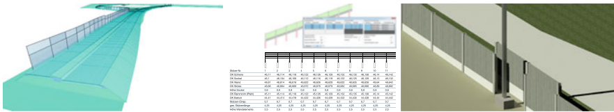
Fig. 34.10 Highway infrastructure modeling (e.g., road layers and noise barrier wall). (© Ed. Züblin AG, reprinted with permission)
