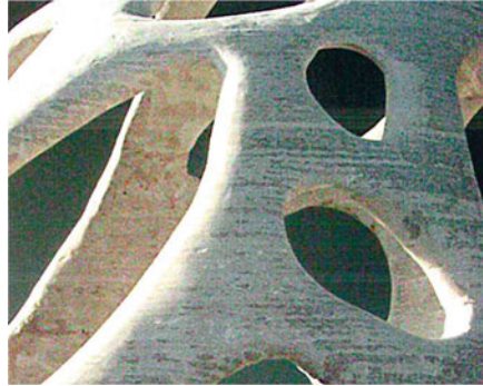
Fig. 26.7 A 3D-printed architectural object made from powder mixture with inorganic solidifying agent. (© Voxeljet AG, reprinted with permission)
