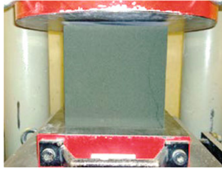
Fig. 26.17 Compression test of an epoxy-infiltrated specimen. (© Ed. Züblin AG, reprinted with permission)
