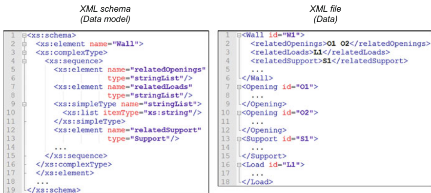
Fig. 3.14 Associations in XML data modeling: binary associations modeled as attributes. Data model (left) and data (right)
