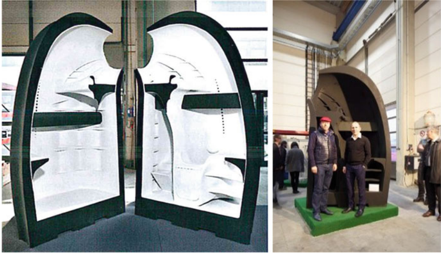
Fig. 26.12 “Micro-home” printed as a sand model; design: Peter Ebner and 3M Future Lab. (© Voxeljet AG, reprinted with permission)
