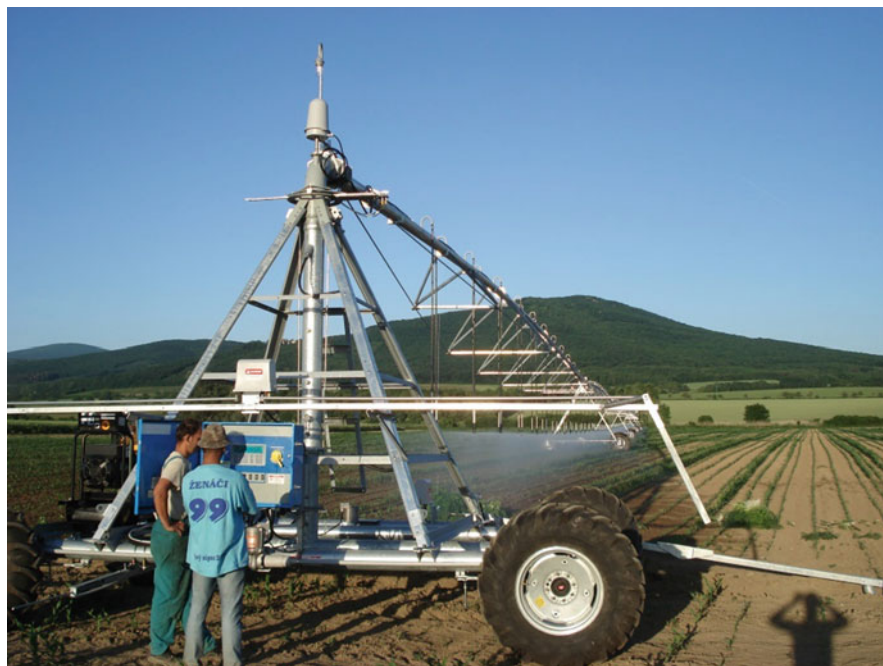
Fig. 4 Linear machine for irrigation at SUA farm Oponice (Photo Jurk 2008)
