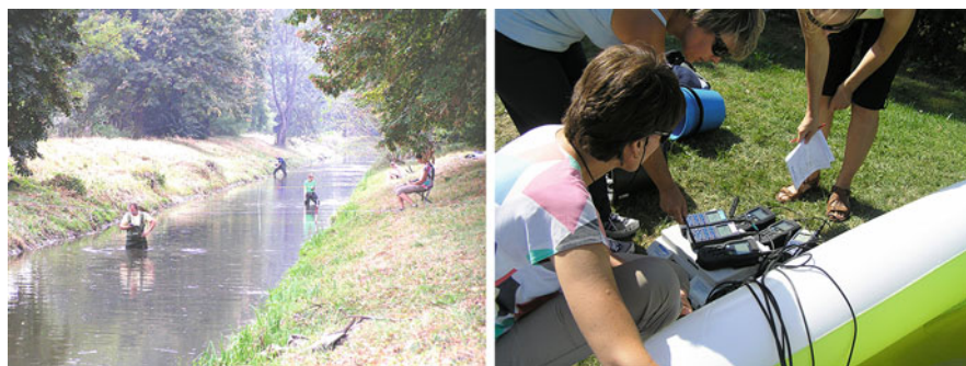
Fig. 17 Measurements along the Malá Nitra stream (measurements of conductivity in cross-section profiles on the left; comparison and calibration of used conductometers on the right)
