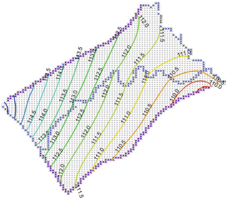
Fig. 11 Course of the groundwater level in the area of interest as of 6.8.2014 – homogeneous environment
