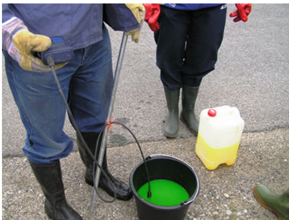
Fig. 12 Tracer preparation, conductivity measurement
