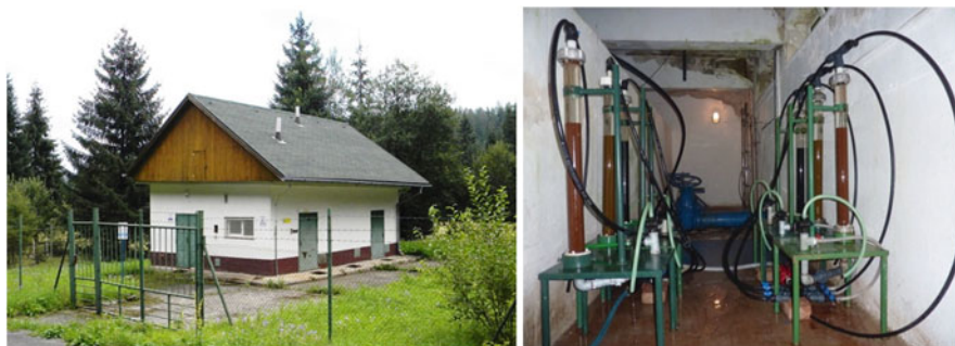
Fig. 5 Dúbrava chlorination plant and model filtration columns
