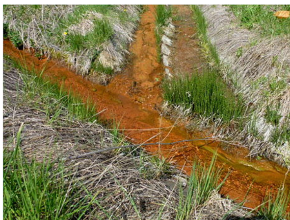
Fig. 9 Outflow of the Sedem Žien setting-pit percolating water from the bottom of the dam (samples V-3 and V-4)
