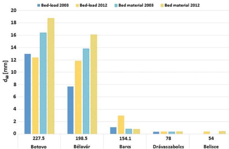
Fig. 7.6 Bedload and bed material grain sizes along the Drava river in 2003 and in 2012
