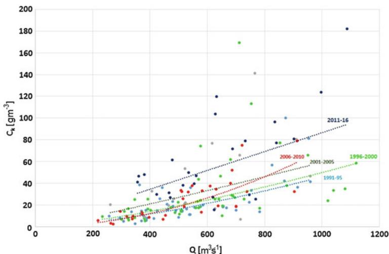
**Fig. 7.8** Suspended load concentration plotted against discharge at Barcs, 1991–2016 ( $n = 164$ ) divided into time periods
