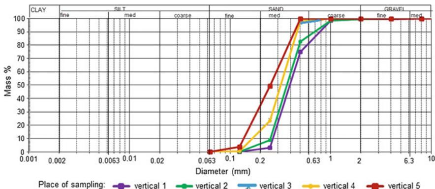
Fig. 7.5 Typical grain size distribution of bed material on the lower reaches (30.08.2012)
