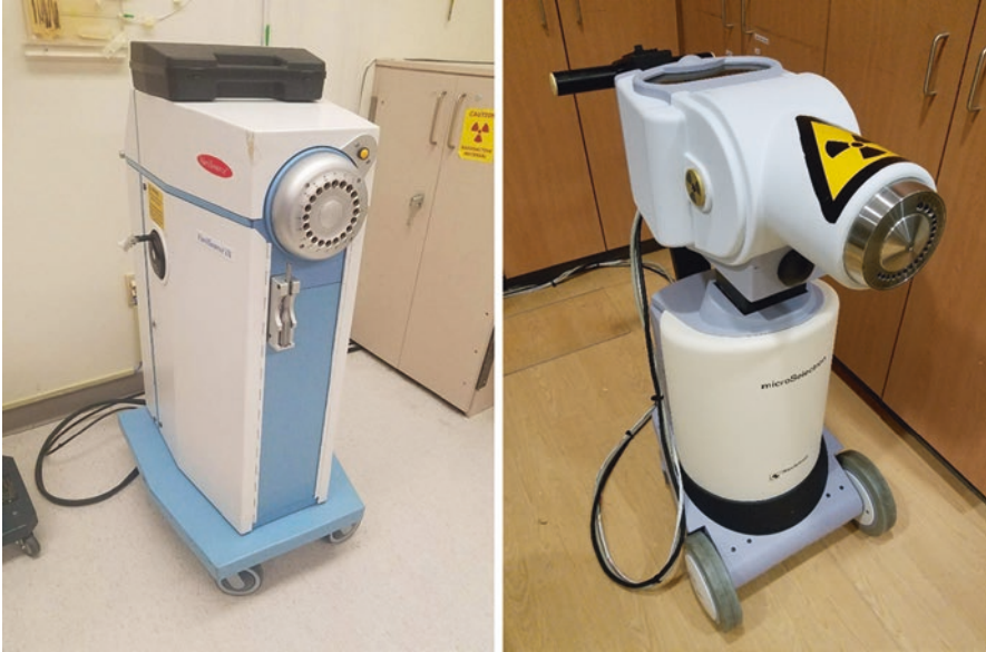
Fig. 2.5 Images of two common remote afterloaders for HDR brachytherapy: Varian Varisource® iX and Elekta MicroSelectron®. Both allow for the controlled placement of a sealed Iridium-192 source into a variety of applicators placed inside/on a patient
