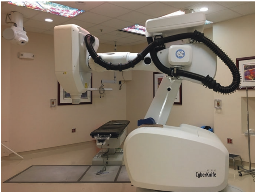
Fig. 2.2 Accuray CyberKnife system with a linear accelerator mounted on a robotic arm. Also shown are the ceiling and in-floor X-ray imaging system and robotic treatment couch
