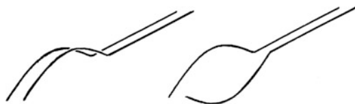
Fig. 4.2 The circulating pulses on the strings when excited in the normal symmetric mode (left) and in the anti-symmetric mode (right)
