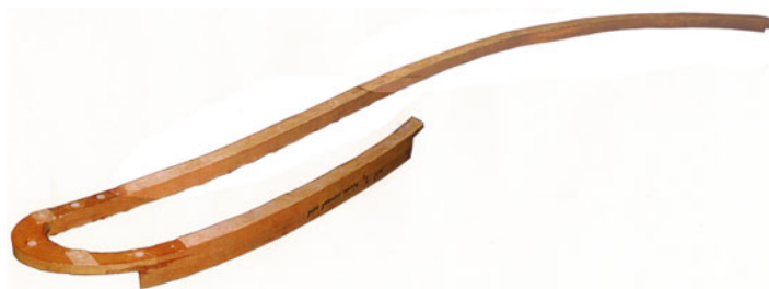
Fig. 4.25 Underside of the compound bridge from a Steinway B grand piano. Note the undercutting in the area where dowels attach the bridge to the soundboard ribs (the four white circles). The bass bridge is at the bottom and a small section of the long treble bridge is at the top (photograph by the author)
