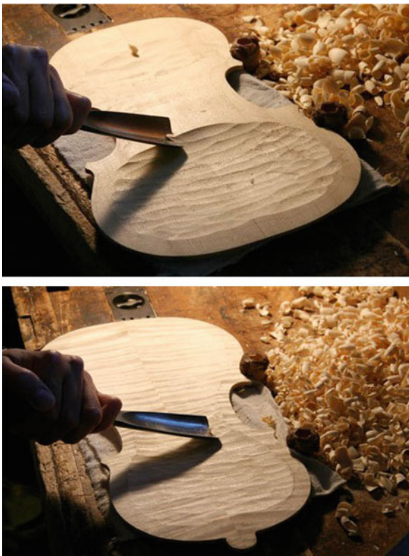
Fig. 5.29 Top (upper) and bottom (lower) plates for a violin being carved by Hiroshi Iizuka. Note the flaming in the bottom plate (photograph courtesy of Iizuka)
