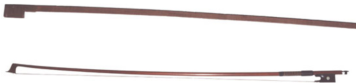
Fig. 5.50 (Top) A piece of pernambuco cut to the rough shape from which a bow can be made. (Bottom) A modern bow fashioned from pernambuco wood by Iizuka (photograph by the author)
