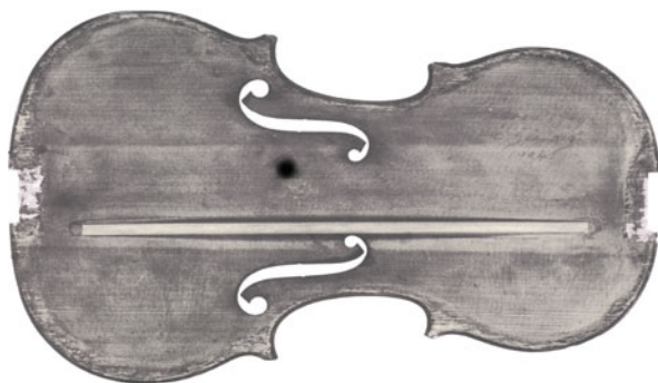
Fig. 5.20 Under-side of a 1709 Stradivari top plate showing the location of the bass bar (long piece of wood at the bottom) and of the sound post. (black circle at the top) (after Sacconi 2000)
