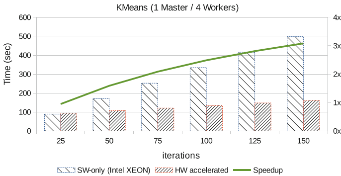
Fig. 5.7 K-means speedup versus the number of the iterations (Intel XEON vs. Pynq)
