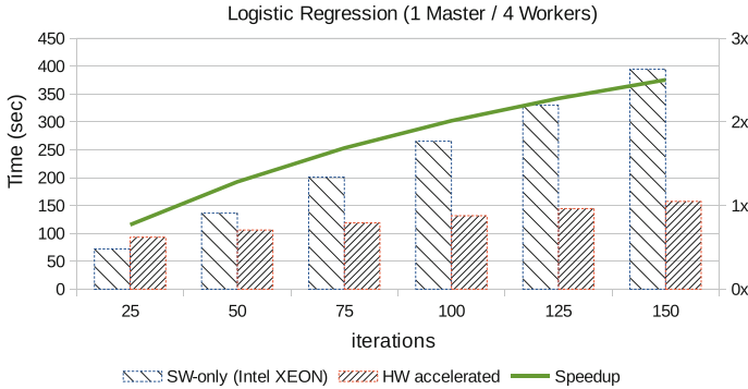
Fig. 5.6 Logistic regression speedup versus the number of the iterations (Intel XEON vs. Pynq)
