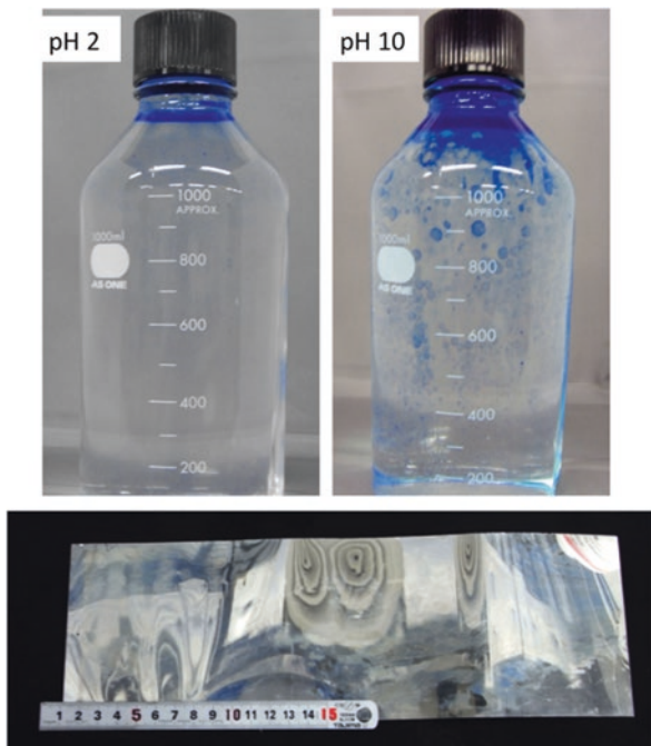
Fig. 1.8 Functionalization of large real life substrates. (Top) 1.3 L glass jar functionalized by low-chemical content SI-ATRP. Jars contain water adjusted to either pH 2 or pH 10 and n -hexane containing blue dye. At pH 2 the surface of the jar was superoleophobic, whereas at pH 10 oil drops adhered to the surface. (Bottom) Aluminum sheet functionalized using SI-“Paint on”-ATRP. (Reproduced with permission from (Dunderdale et al. 2014), Copyright 2014 The American Chemical Society)
