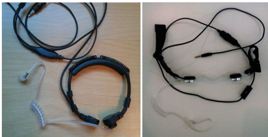
Fig. 15.5 Throat-microphones used in [182]. (Reprinted with permission from IEEEACM Transactions on (T-ASL) Audio, Speech, and Language Processing)
