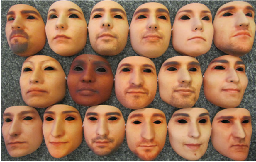
Fig. 9.3 Example of 3D masks. These are the 17 hard-resin facial masks used to create the 3DMAD dataset, from [13]
