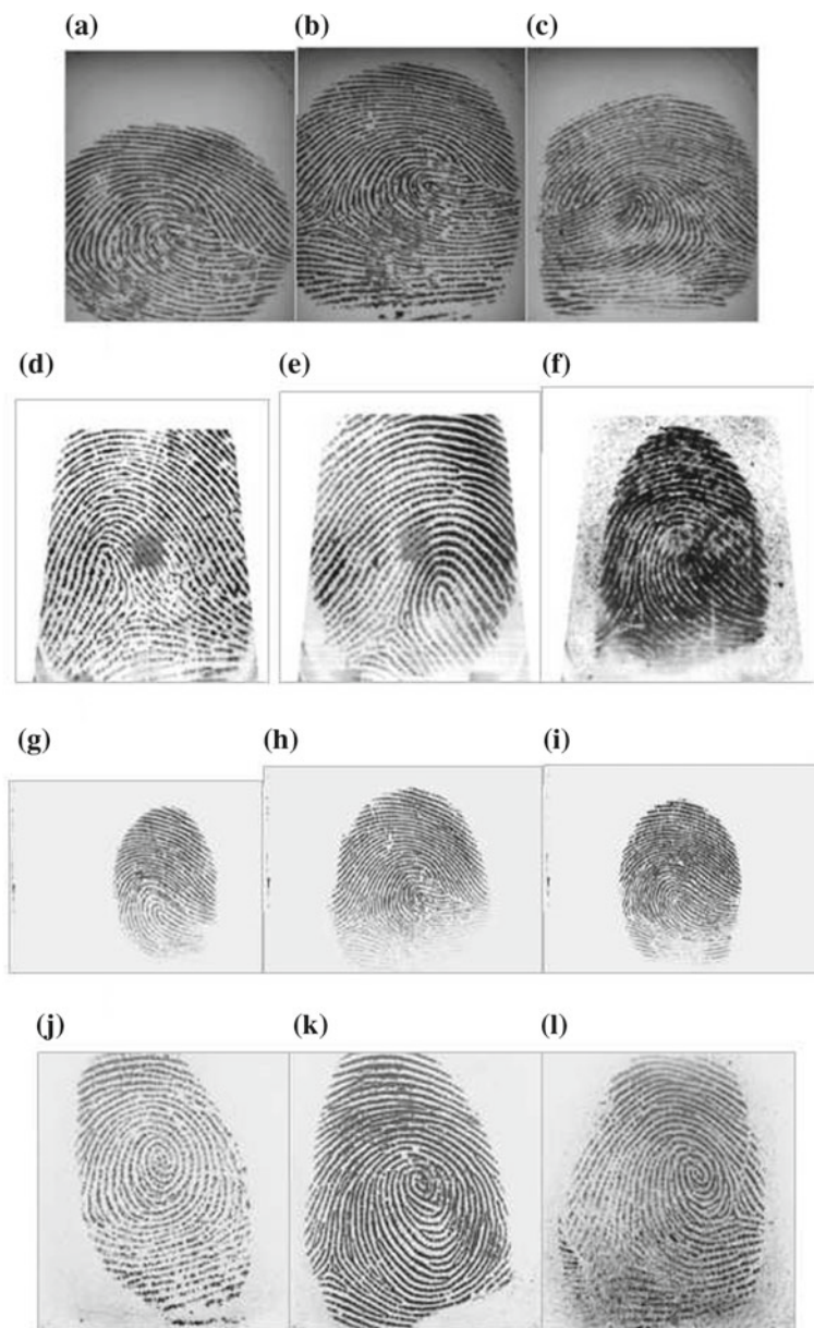
Fig. 5.2 Examples of fake fingerprint images of the LivDet 2011 datasets, from Biometrika a latex, b gelatin, c silicone; from Digital Persona: d latex, e gelatin, f silicone; from Italdata: g latex h gelatin i silicone; from Sagem: j latex k gelatin l silicone
