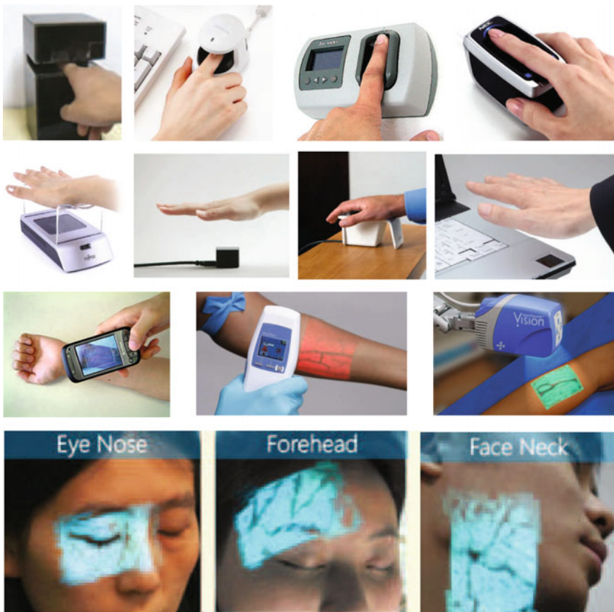
Fig. 18.2 Examples of commercial vein sensors, first line finger vein sensors, palm vein sensors, and the last two lines show medial vein sensors
