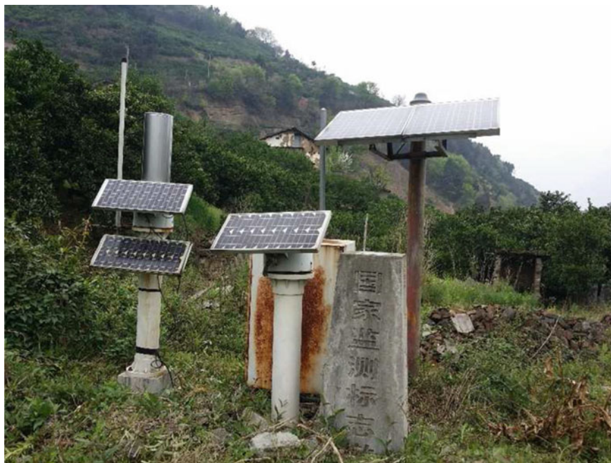
Fig. 3.5 Detecting rain gauge and deep deformation
