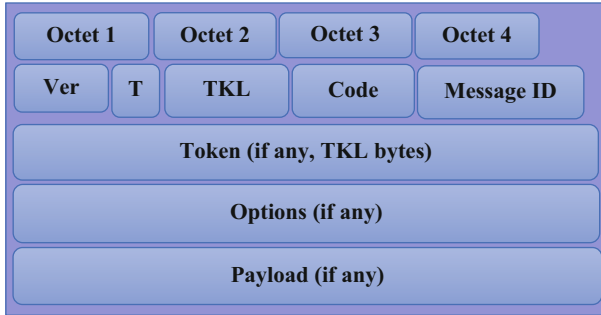
Fig. 7.6 Constrained Application Protocol (CoAP) message format
