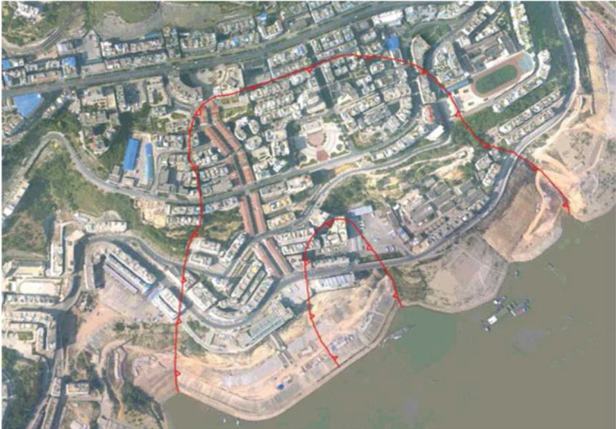
Fig. 3.2 Identify a landslide from remote sensing images
