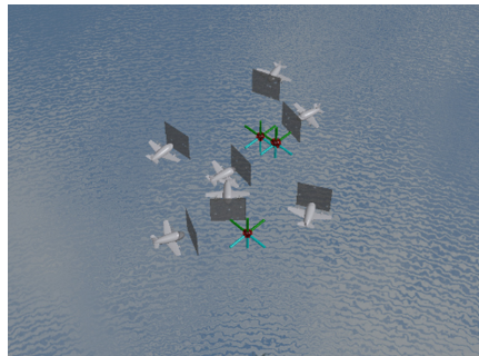
Fig. 6. Frame 500 with realistic rendering. Three axes are the targets and red balls are EKF trackers. (Color figure online)
