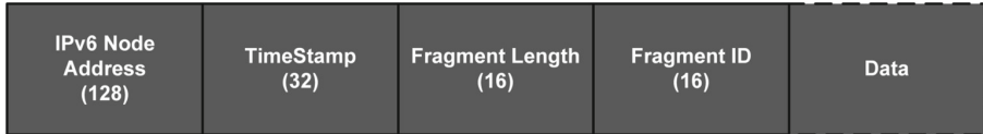
Fig. 3. The structure of the data placed in the Monitoring Header by the node. In parentheses is the length of the data fields in bits.
