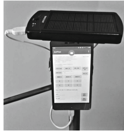
Fig. 7. Wireless node with solar panel and the management application
