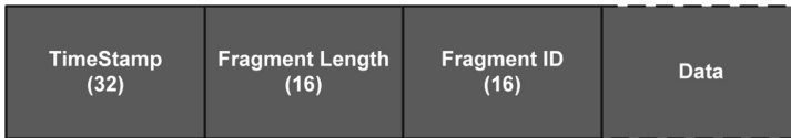
Fig. 1. The data structure placed in a package by the monitored node. In parentheses is the length of the data fields in bits.
