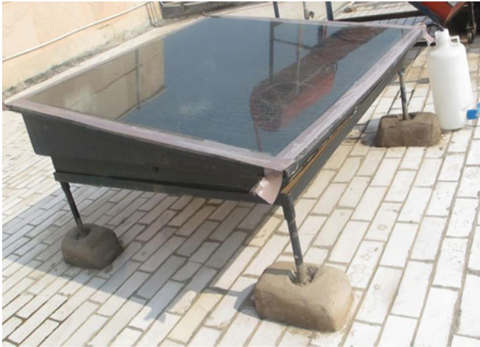
Fig. 3 Single slope, single basin-type solar still with distillate collector [7]
