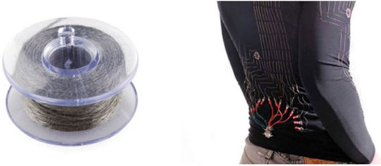
Fig. 5 Conductive thread used to create embedded electronics within clothing
