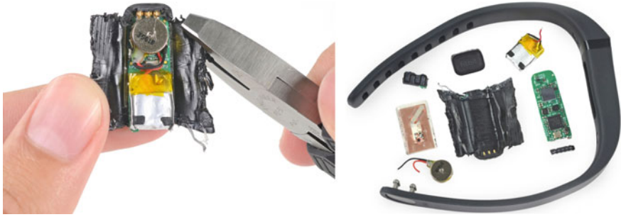
Fig. 10 Fitbit Flex teardown process [34]
