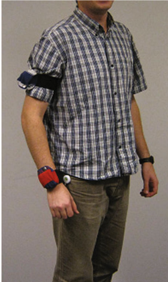
Fig. 2 A male subject wearing two body surface sensor nodes, the first sensor at the right wrist and the second sensor at the upper left arm [6]
