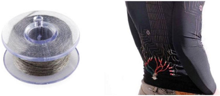
Fig. 5 Conductive thread used to create embedded electronics within clothing
