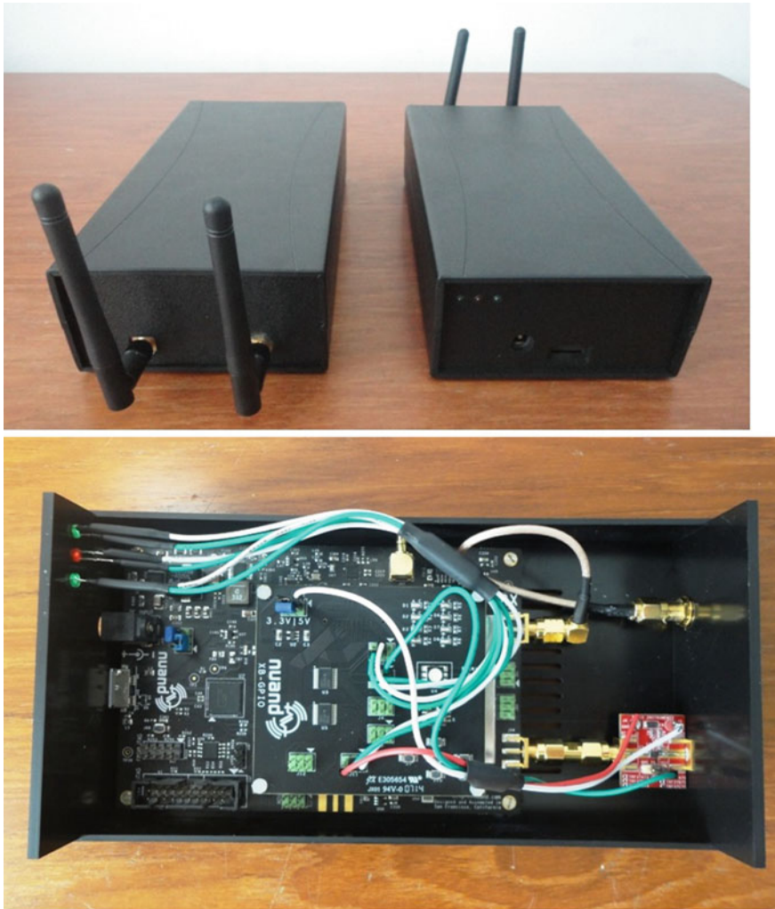
Fig. 14 An SDR platform from Nuand was used to build the fully autonomous cooperative routing scheme. The platform houses a 40-KLE Altera Cyclone IV FPGA, a Cypress microcontroller unit (MCU), and a reconfigurable RF chipset from Lime Microsystems. An RF amplifier from Texas Instruments was also annexed to the platform. The OFDM PHY was built on the FPGA, while the rest of the protocol stack runs on the MCU
