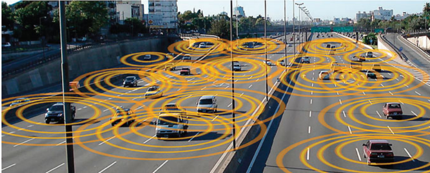
Fig. 1 Cooperative safety systems, such as CCW, rely on the broadcast of vehicle movement information over a local wireless network
