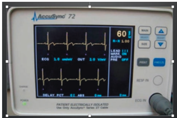
Fig. 12.2 Interface for the synchronization of the irreversible electroporation pulses with the refractory period of the cardiac rhythm
