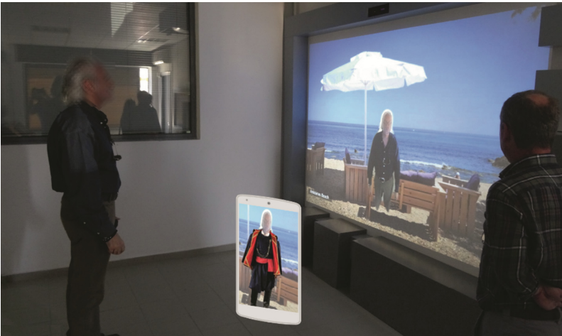
Fig. 4. View of the AR application on a mobile device as a user assigns an element to follow user’s movement in the MR display
