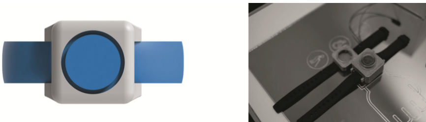
Fig. 3. Render and prototype of the wearable band
