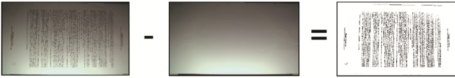
Fig. 6. Image difference process (the last image already limiarized) (Color figure online)
