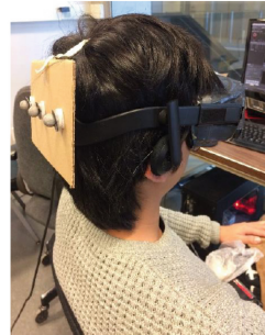
(b) Oculus VR setup with 3 head-mounted IR markers
