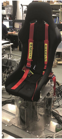
Fig. 1. A vestibular display (motion seat) of three degrees of freedom (lift, roll, pitch motion)
