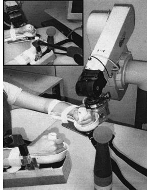
Fig. 1. Robot-Assisted training through MIME. [9]
