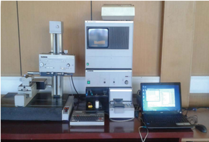
Fig. 1. Surface roughness measurement system Talysurf-6 connected with computer
