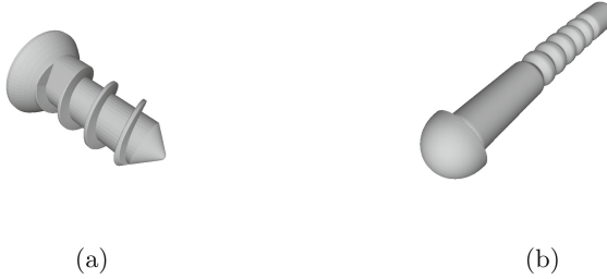
Fig. 2. Surgical instrument models: (a) Screw - 6 DoF model (position and orientation) and (b) Robot - 8 DoF model (position, orientation and joint configuration)
