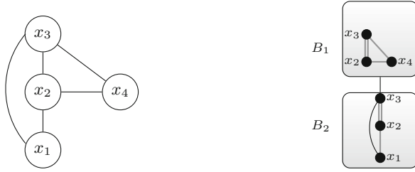
Fig. 1. On the left a constrained graph representing the Formula \{\{x_1, x_2\}, \{x_1, x_3\}, \{x_2, x_4\}, \{x_2, x_3\}, \{x_3, x_4\}\} . On the right, its tree decomposition.
