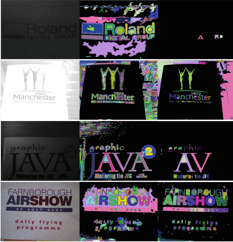
Fig. 4. Synthetic degradations. From up to down: low contrast, high brightness, nonuniform illumination, and additive noise. From left to right: degraded image, proposed method result, and MSER method result.
