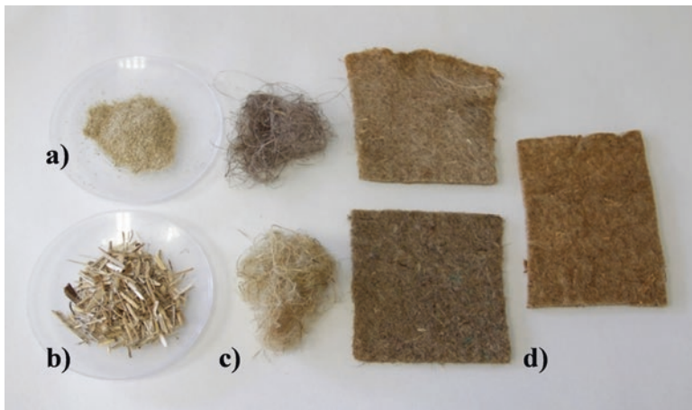
Fig. 1.6 Pictures of the hemp-based materials used as biosorbents: (a) sawdust, (b) hurds (shives), (c) fibres and (d) felt
