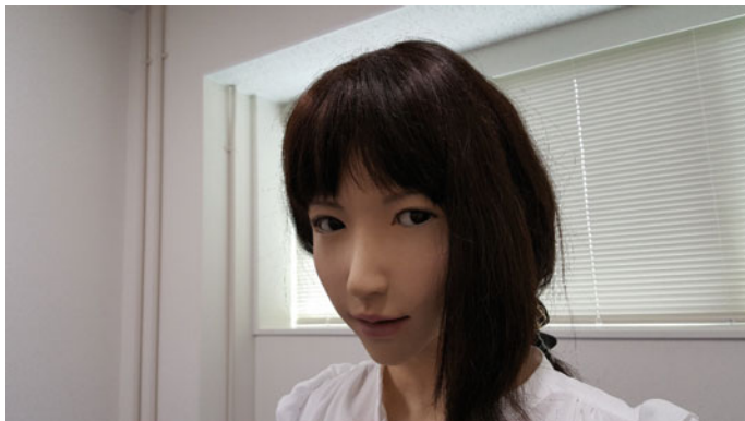
Fig. 1 The android Erica is designed to be physically realistic. Motors within her face provide speaking motions in addition to unconscious behaviors such as breathing and blinking
